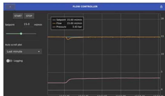
Flow Control mode - Increased or reduced back pressure is compensated automatically
