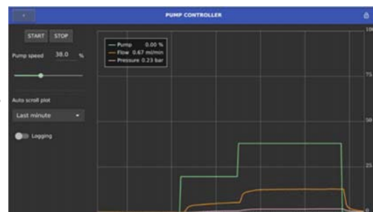
Pump Control mode - Pump speed can be controlled between 0 and 100%
